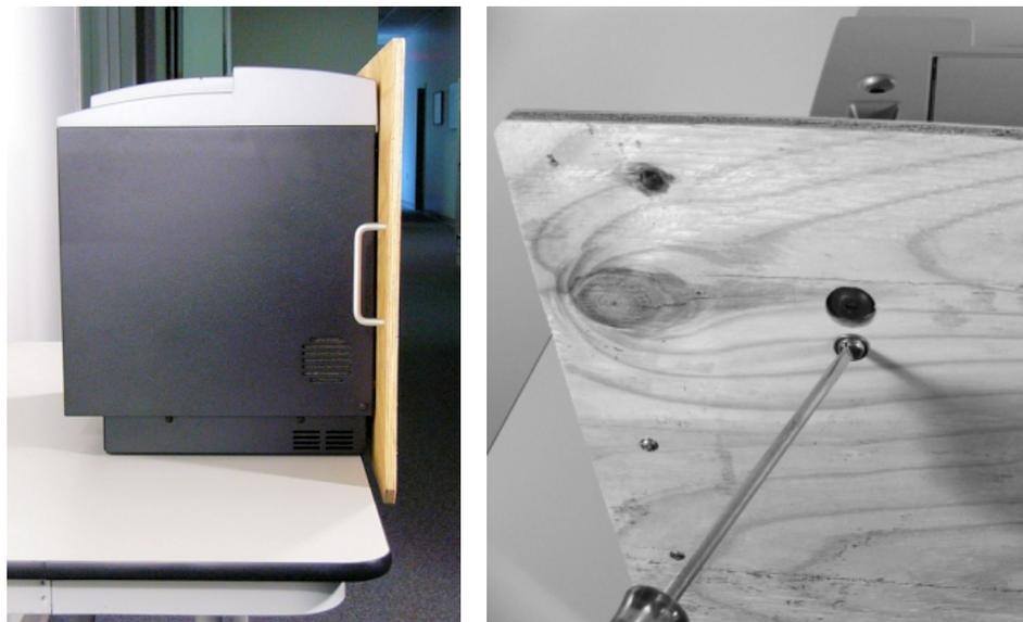
Figure 2-1: The reader on its back with the shipping panel attached to the bottom (left), and removing the screws (right)
