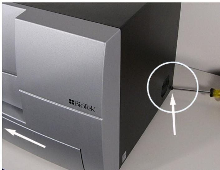
Figure 2-2: Locating and removing the two side screws
