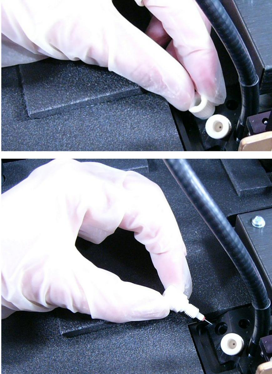
Figure 5-4: Removing the injector heads
