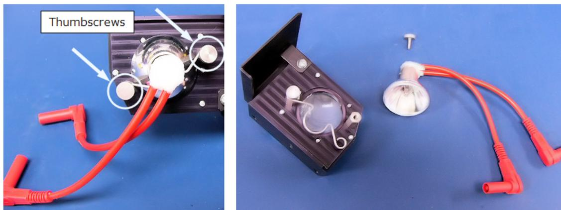
Figure 6-2: Removing the old bulb (with cables) from the bracket
