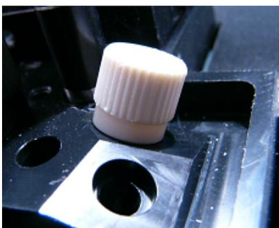
Figure 5-13: Seating the injector head
