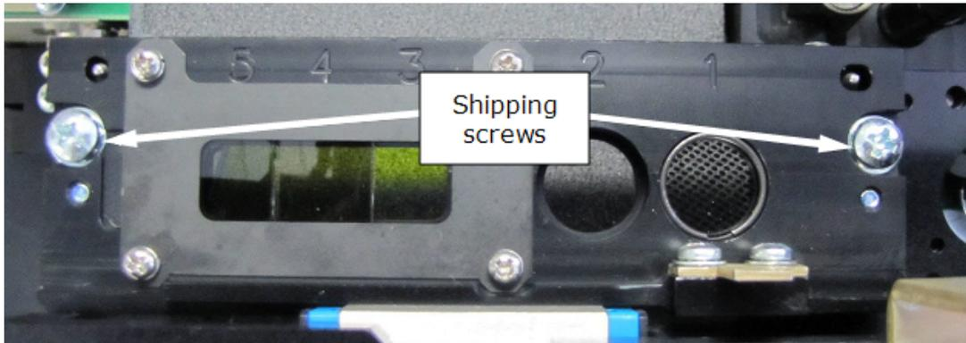
Figure 2-10: Mirror holder shipping screws
