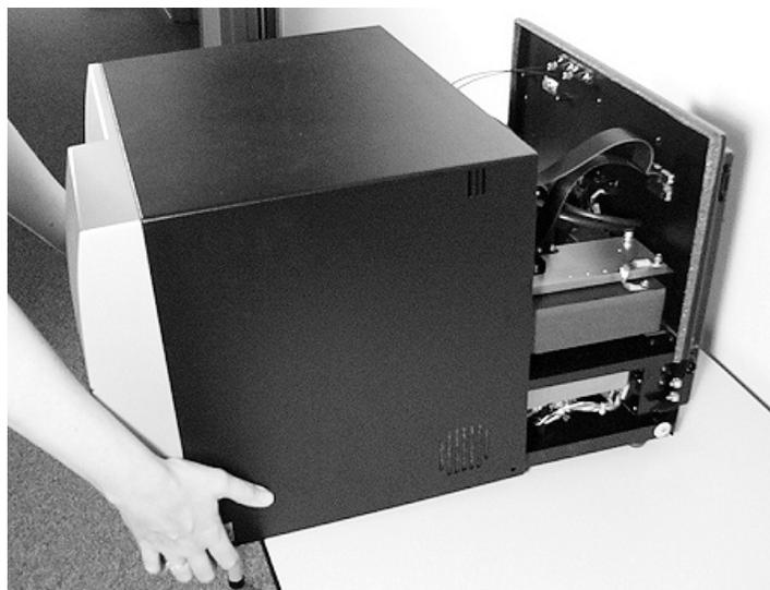
Figure 2-3: Sliding off the shroud
