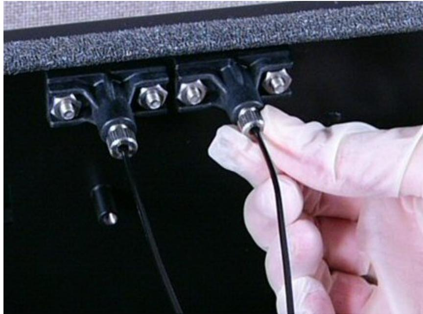
Figure 5-2: Disconnecting the dispense tubes from the back wall
