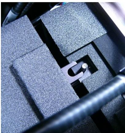
Figure 5-12: Positioning the incubator housing fork
